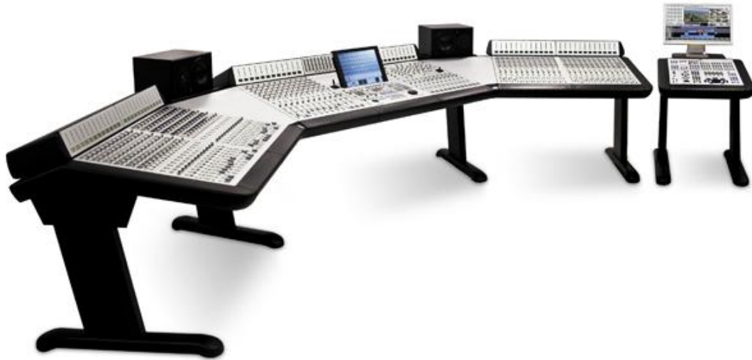
Anthem 240 channel large format mixing powered by a single CC-1 card.
